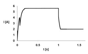
Figure 1: Typical current consumption using the ADRV1003W000399 with a 4 Ohm solenoid at 24V DC supply voltage.
