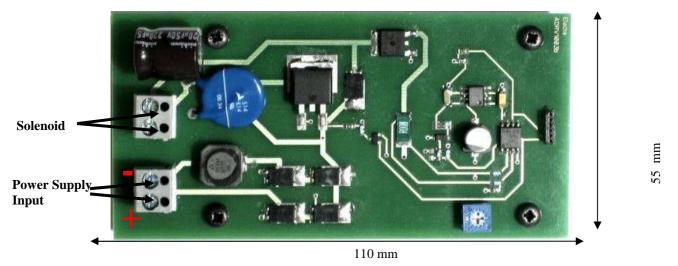
Figure 2: Connection schematic and dimensions, top view. The polarity for the DC version is indicated in red
